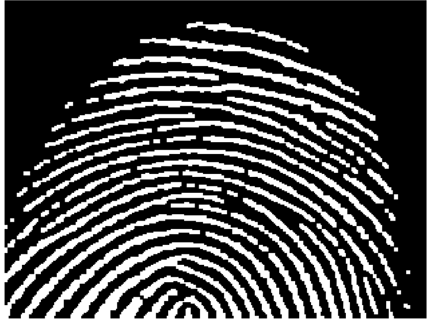
Image after segmentation and morphological processing
